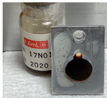
Fig. 2. Photograph of the sample container and the sample of Resovist.
