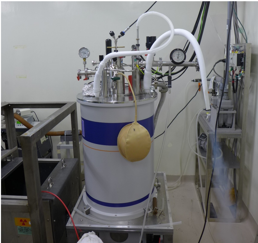
6T superconducting magnet for Mössbauer Spectroscopy
