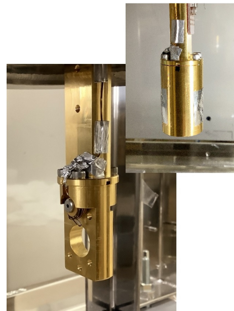
Fig. 2. Photo of the sample stage (Au plated).
