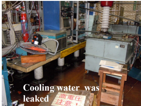
Fig.10 The flooded polarized ion source due to the broken water pressure gauges of the cooling water system.
