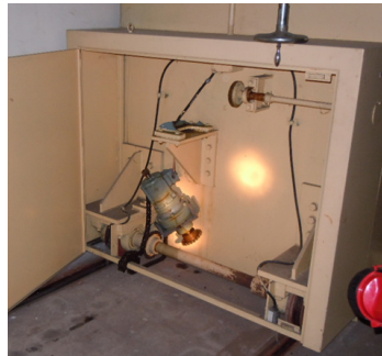
Fig.17 Broken shielding door motor at the analyzer magnet room.
