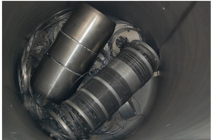
Fig.15 Photo of the fallen terminal shell and accelerator columns at the tank bottom.
