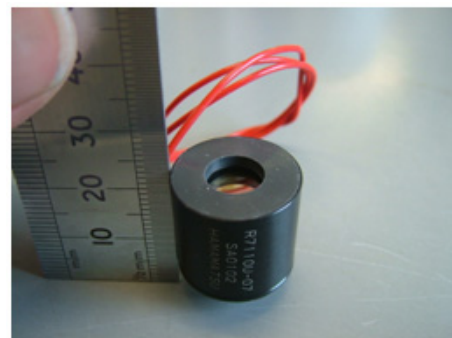
Fig.2. HPD (HAMAMATSU R7110U-07) that we used in this experiment.
